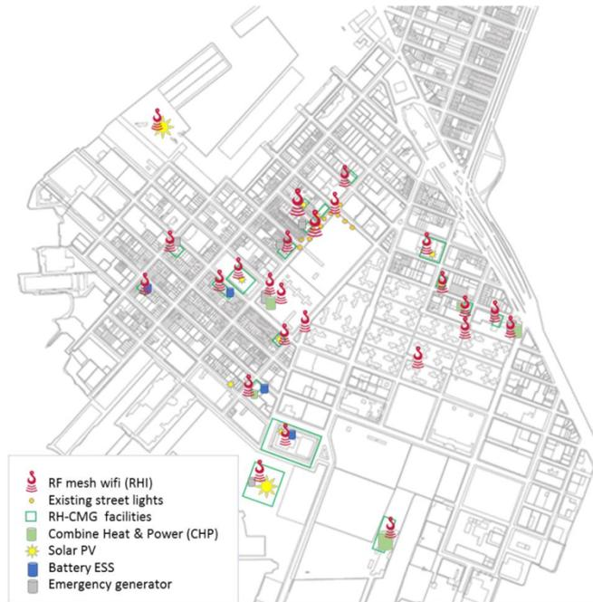
**Figure 9: RH-CMG Communications Nodes – RHI RF Mesh**
