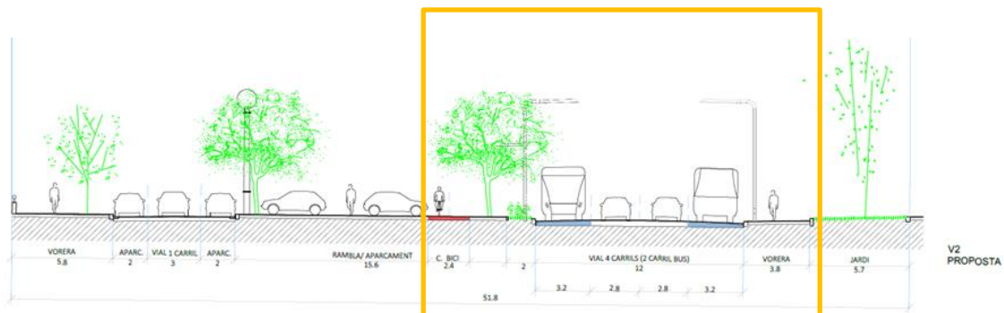
C-245 road section 50 m-wide in Viladecans after with 3.2m- bus lanes and a 2.4m bike lane © Generalitat de Catalunya, DeSola-Gori Architects (March 2018)
