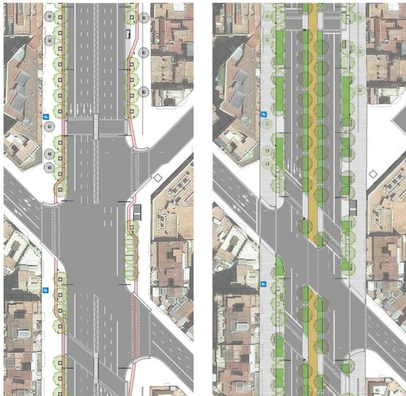
Section 2. Before (left) and after (right) where two traffic lanes are removed, a central bikeway and two more rows of trees are created (north is at top)
