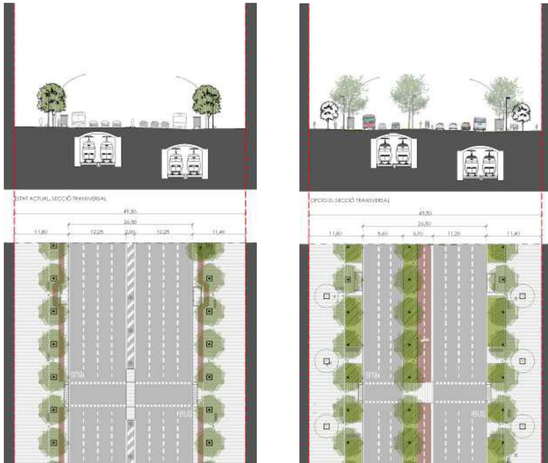
Cross sections of a typical section of the Meridana before (left) with 4+4 traffic lanes (including 2 bus lanes) and after with a narrow median for a bike lane and 4+3 traffic lanes including 2 bus lanes (right) © Ajuntament de Barcelona
