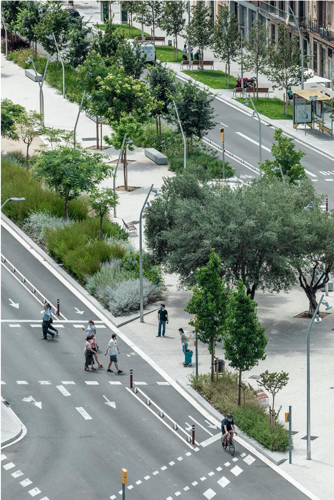
Between Plaça de les Glories and Arago street, the Meridiana layout, designed with SBS Simón i Blanco (engineers) and Batlleiroig (architects & landscape architects), features a large shaded promenade with trees serving as a refuge for birds and flower gardens attracting butterflies. Notice the large and comfortable pedestrian crossings and the quality of the design. The bike lane is along the roadway here (it is integrated into the central rambla further north)
